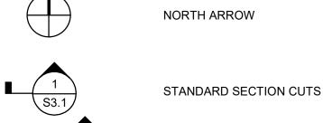
1 S3.1 **BUILDING SECTION CUTS** ELEVATION OF WALL OR FRAME
