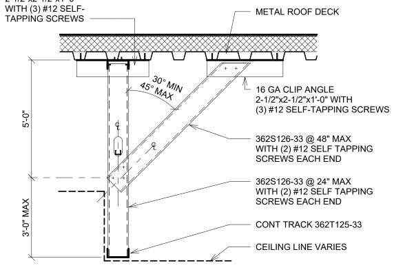
BULKHEAD DETAIL - PARALLEL TO ROOF DECK
