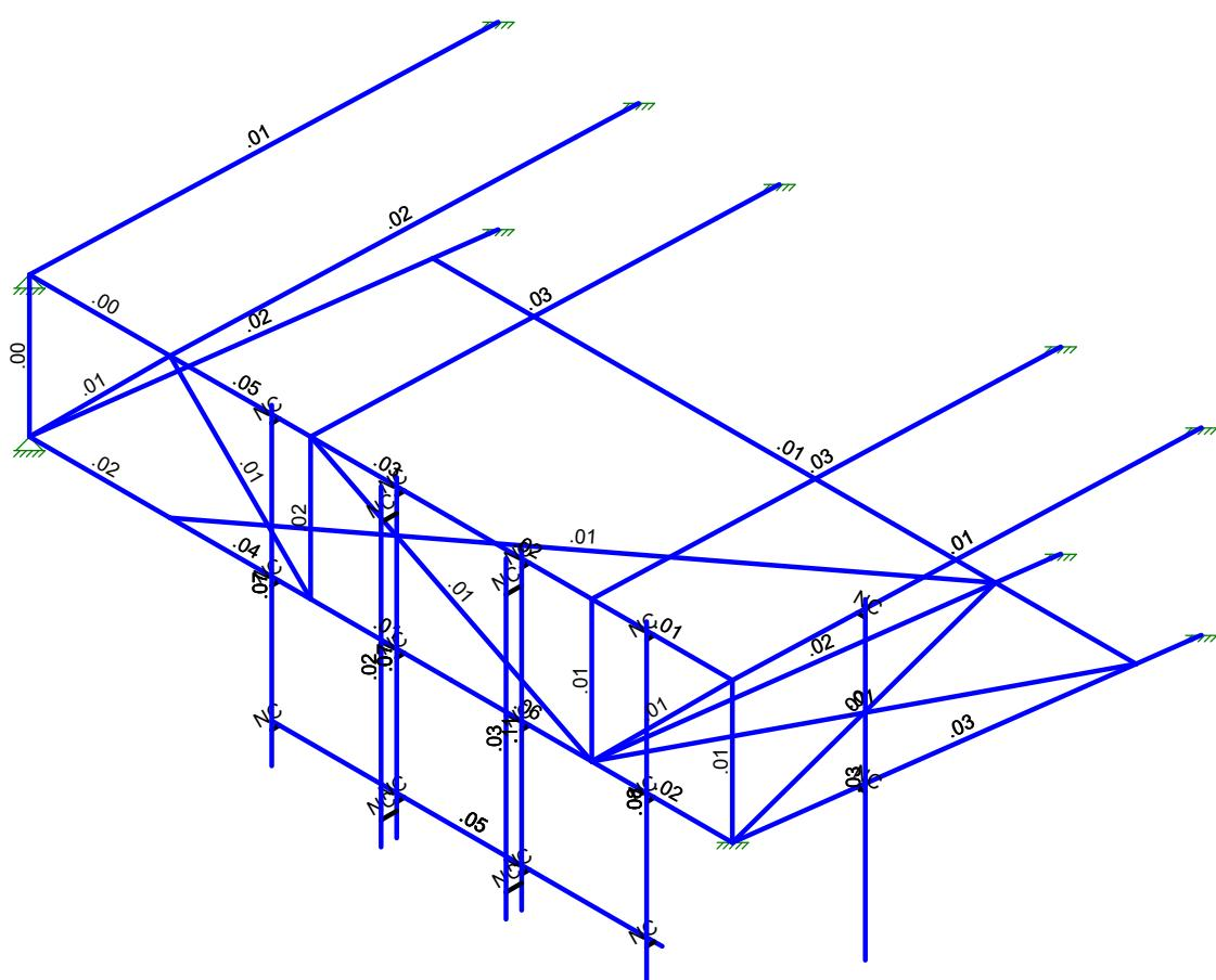
Member Shear Checks Displayed (Enveloped)
