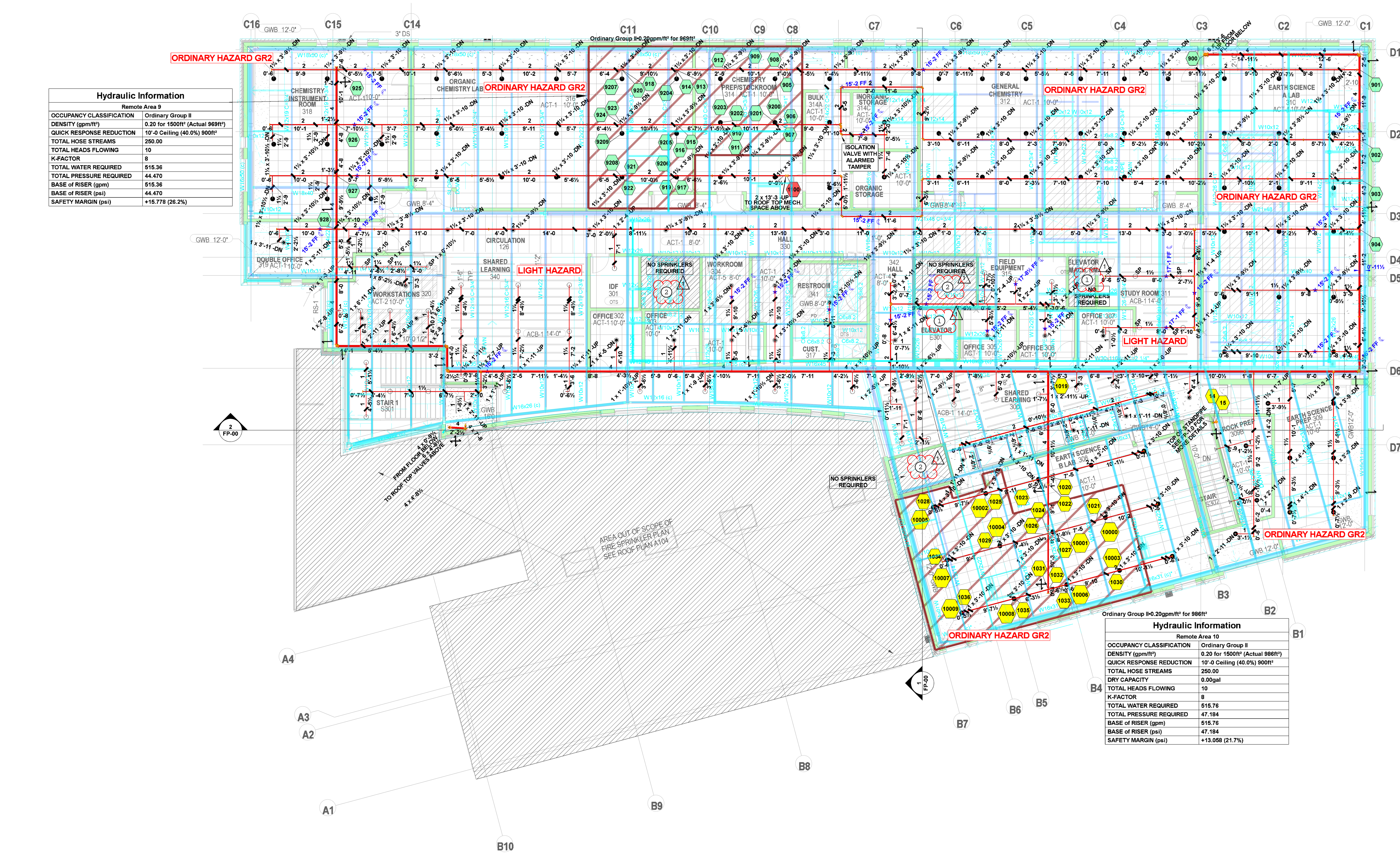
FIRE SPRINKLER PLAN - THIRD FLOOR SCALE 1/8"=1'-0"
