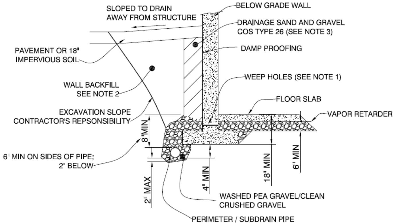
1. Washed pea gravel/crushed rock beneath floor slab could be hydraulically connected to perimeter/subdrain pipe. Use of 1" diameter weep holes as shown is one applicable method. Crushed gravel should consist of 3/4" minus. Washed pea gravel should consist of 3/8" to No. 8 standard sieve.
