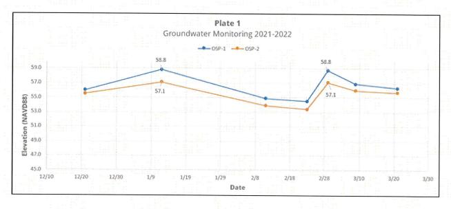
We anticipate fluctuations in the local groundwater levels will occur in response to precipitation patterns, off site construction activities, and site utilization. As such, water level observations made at the time of our field investigation may vary from those encountered during the construction phase. Analysis or modeling of anticipated groundwater levels during construction is beyond the scope of this report.
