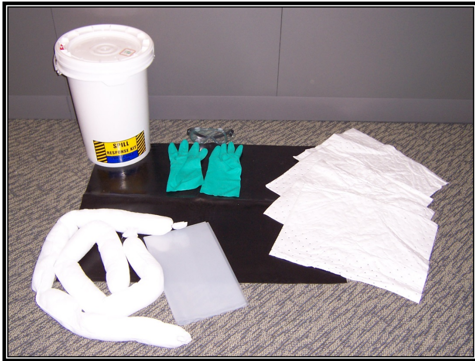
Figure 4.25. Example of Spill Kit Contents.
