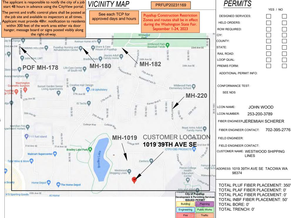
NARRATIVE: THIS PROJECT WILL PROVIDE CDFS SERVICE TO 1019 39TH AVE SE . EXISTING 48 FIBER CABLE FROM MH-178 TO MH-180 IN EXISTING CONDUIT.EXISTING 48 FIBER CABLE FROM MH-180 TO MH-182 IN EXISTING CONDUIT.EXISTING 24 FIBER CABLE FROM MH-182 TO MH-220 IN EXISTING CONDUIT.PLACE NEW 24 FIBER CABLE FROM MH-220 TO MH-1019 IN THE EXISTING CONDUIT.CONTINUE NEW 24 FIBER CABLE FROM MH-1019 TO CUSTOMER MPOP IN EXISTING CONDUIT.
