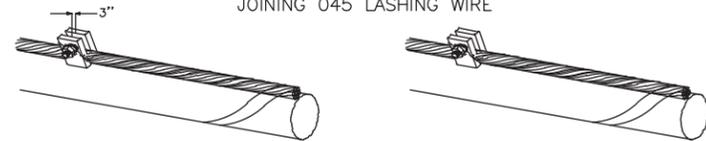
REMOVE ANY SLACK IN THE LASHING WIRE BY MAINTAINING A PULL ON THE WIRE AND TAPPING THE STRAND SHARPLY. THEN FORM THE WIRE OVER THE STUD AND TIGHTEN THE NUT. CUT THE FREE END OF THE LASHING WIRE OFF 3/4" BEYOND THE END OF THE CLAMP.
