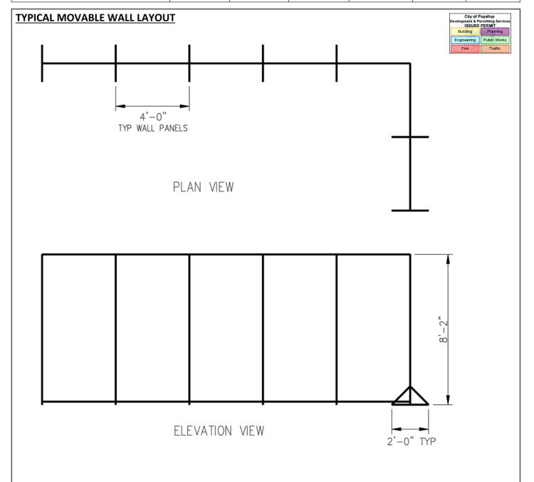
ASSUME EVERY OTHER T-LEG SUPPORT IS ANCHORED TO CONCRETE FLOOR → 8'-0" o/c
