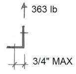
$$\begin{split} M_{PL} = 363 \text{ lb} \times 0.75 \text{ in } / & 2 = \textbf{0.136} \text{ kip\_in} \\ M_n = F_y \times 2.75 \text{ in} \times & (0.0516 \text{ in})^2 / 4 = \textbf{0.060} \text{ kip\_in} \\ M_{PL} > & M_n \quad 18 \text{ GA ANGLE FAILS} \end{split}$$
