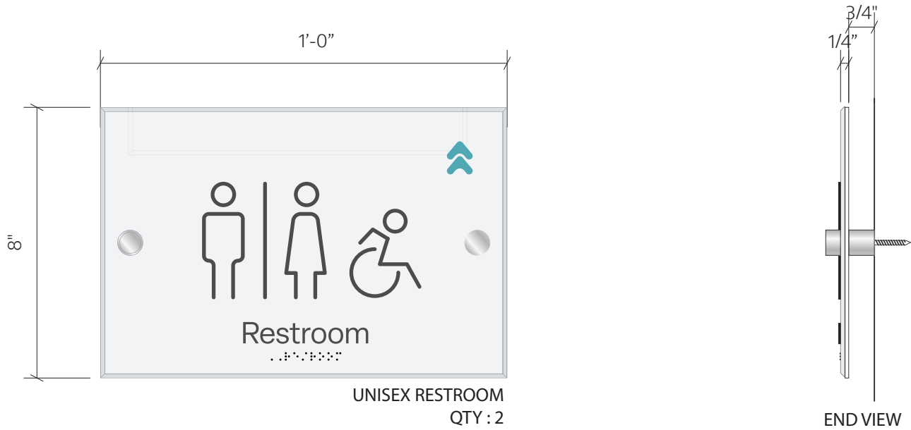
P20 UNISEX RESTROOM ADA SIGN UB-ADA-RR-PANEL-C SCALE : 3"=1'-0" 0.66 SQ.FT COLOR SPECIFICATION TO MATCH 3M # 220-41 - DARK GREY
