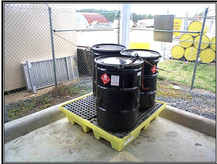
Figure 4.17. Temporary Secondary Containment.
