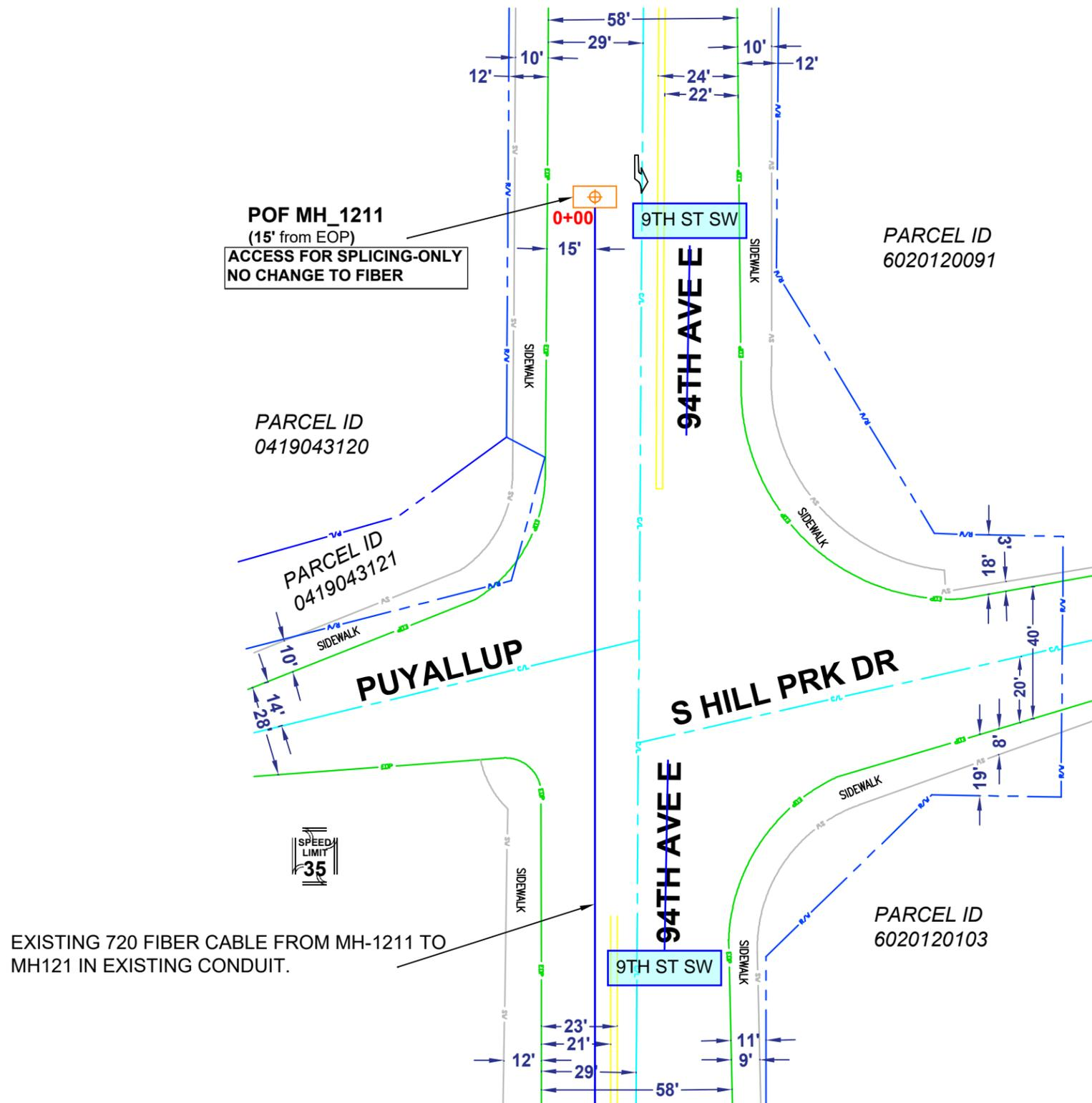
EXISTING 720 FIBER CABLE FROM MH-1211 TO MH121 IN EXISTING CONDUIT.
