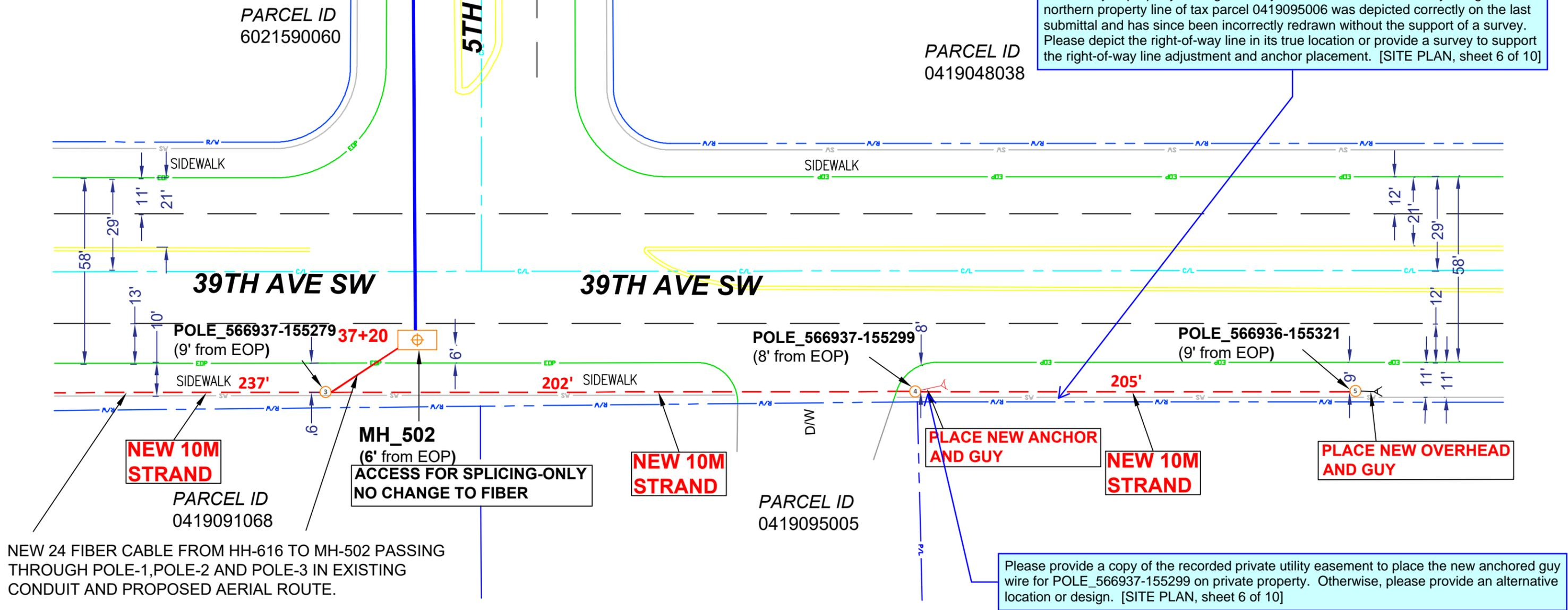
NEW 24 FIBER CABLE FROM HH-616 TO MH-502 PASSING THROUGH POLE-1, POLE-2 AND POLE-3 IN EXISTING CONDUIT AND PROPOSED AERIAL ROUTE.
