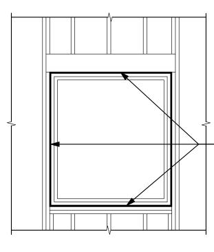
INSTALL CONTINUOUS BACKER ROD AND SEALANT AT HEAD, JAMBS, AND SILL (INTERIOR SECONDARY SEALANT JOINT, AIR BARRIER)
