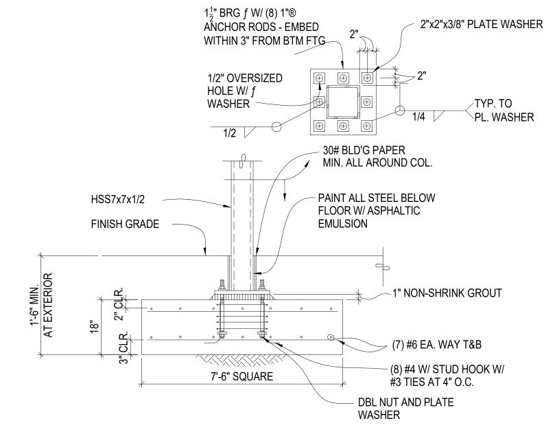
5 TYPICAL STEEL COLUMN ON SPREAD FOOTING
