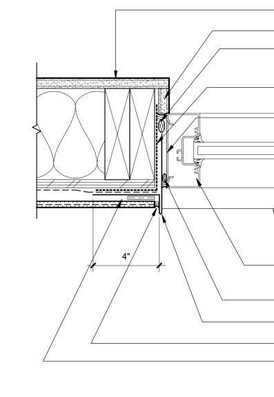
THRESHOLD BELOW STOREFRONT PER SCHEDULE ALIGN FACE OF FRAME WITH FACE OF SHEATHING BACKER ROD AND SEALANT, TYP, EA. SIDE PREFINISHED SHEET METAL JAMB FLASHING SEALANT MATCH DEPTH RELATIVE TO FRAMING AS VERTICAL FLASHING
