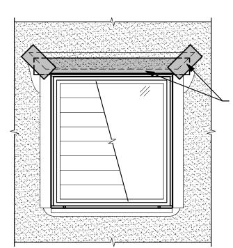
FLIP HEAD FLAP DOWN AND TRIM 1" - 2" ABOVE WINDOW OPENING, TERMINATE FLAP ALONG THE TOP OF WINDOW WITH TAPE; TAPE DIAGONAL CUTS WITH SELF-ADHERED FLASHING AND ROLL DOWN TIGHT TO ACHIEVE PROPER ADHESION USING A 2-HANDED ROLLER AND HEAVY PRESSURE
