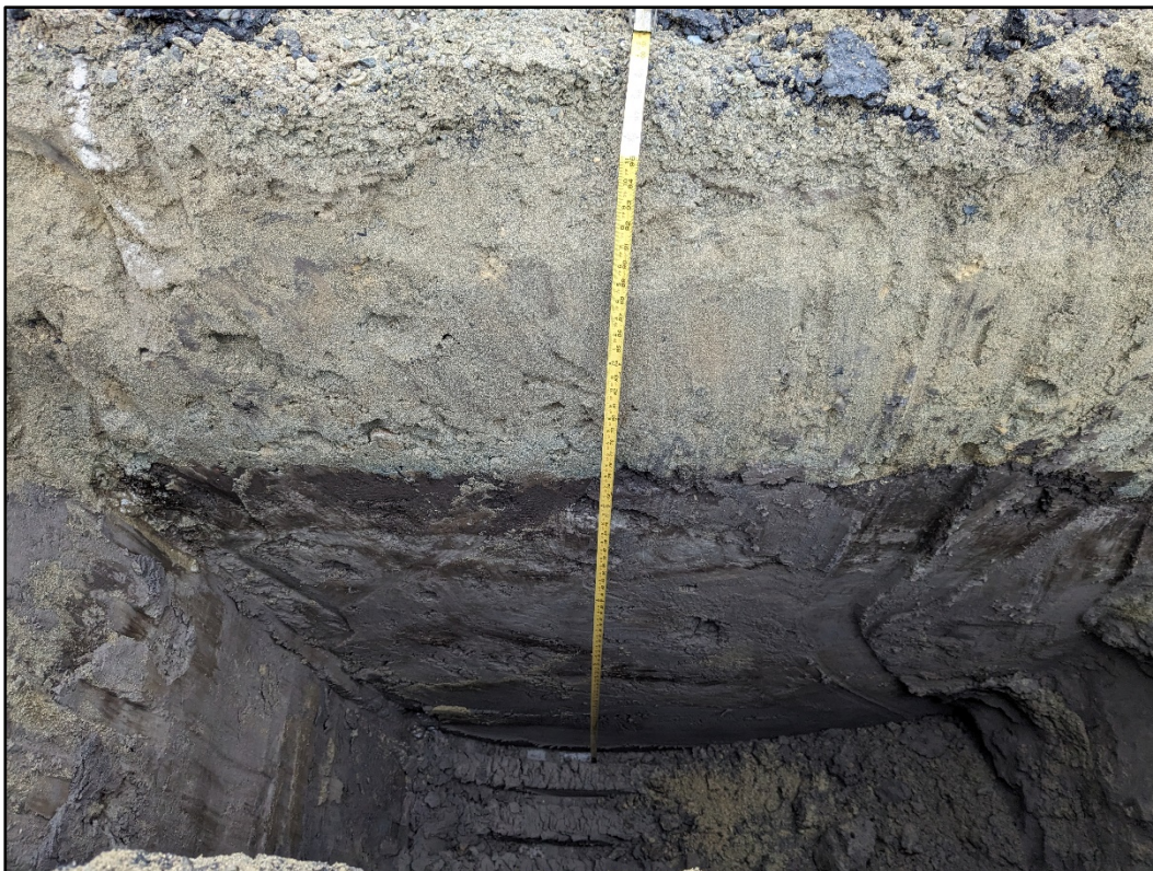
Figure 11. Overview of TT-6 showing typical profile of sandy fill over alluvium.
