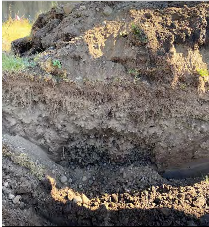
Plate 1. Sidewall view of TP-1. Previous aggregate pier seen about 1 foot below grade.
