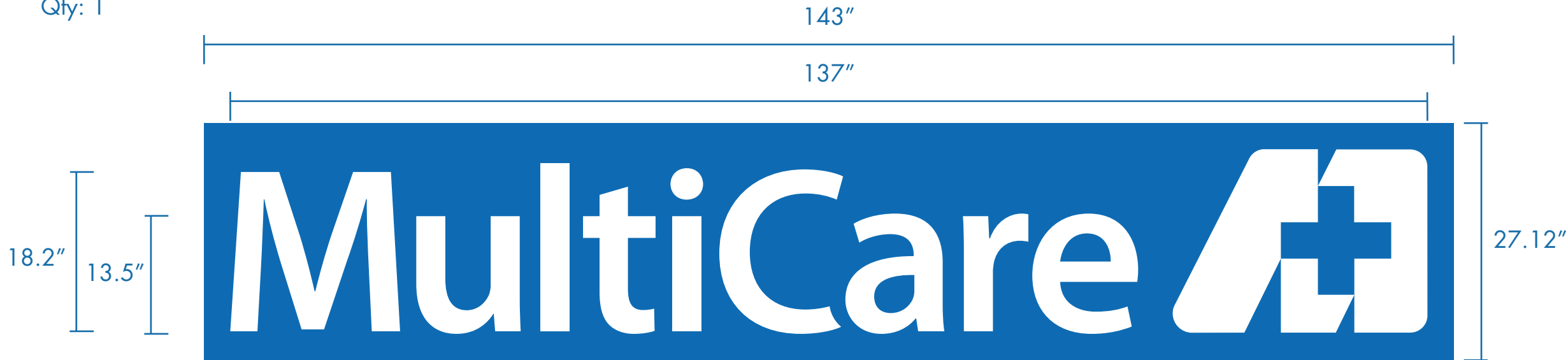
FRONT VIEW (SCALE 1:14) SIGN AREA: 190 SQ. FT OVERALL WEIGHT OF THE SIGN: 400 LBS.
