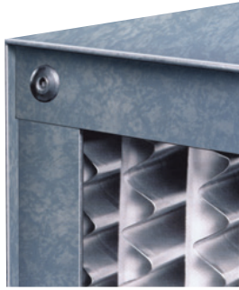
Crimped Rear Flanges (SH) are rolled over and riveted to add strength, eliminate sharp edges, and prevent bypass leakage.
