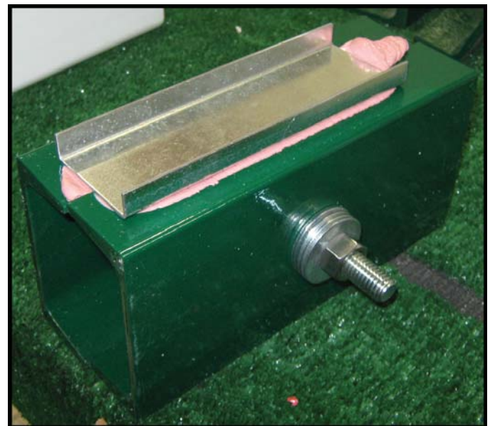
Press split cover down over the center of the caulking until caulking seeps out of both sides of cover.
