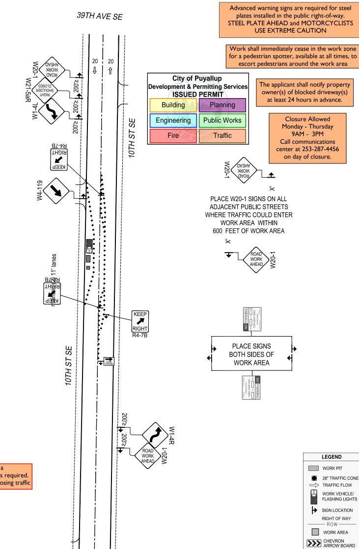
When shifting traffic into a turn lane the use of double cones is required. Device spacing 1/2 distance for opposing traffic
