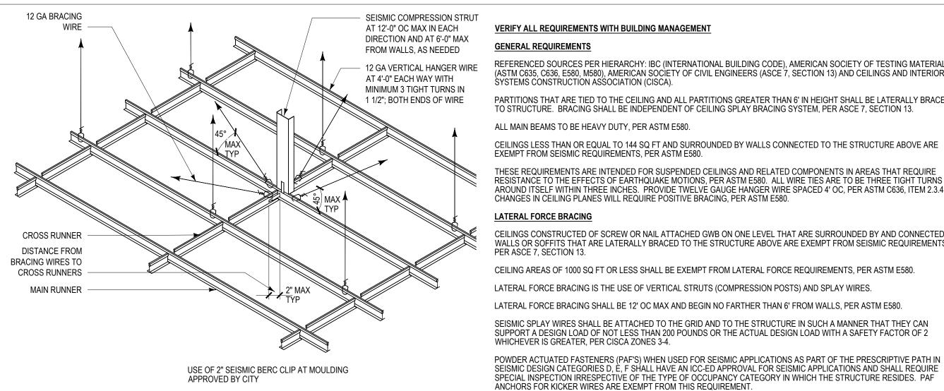
PROVIDE ACT SUSPENSION GRID TO COMPLY WITH IBC SECTION 1613 MINIMUM STANDARD: ASTM C636, ASTM E580, ASCE 7, SECTION 13; REF NOTES
