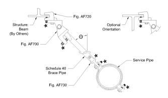
\* - denotes hardware shown with the bolt head or nut broken off, as per the product installation instructions
