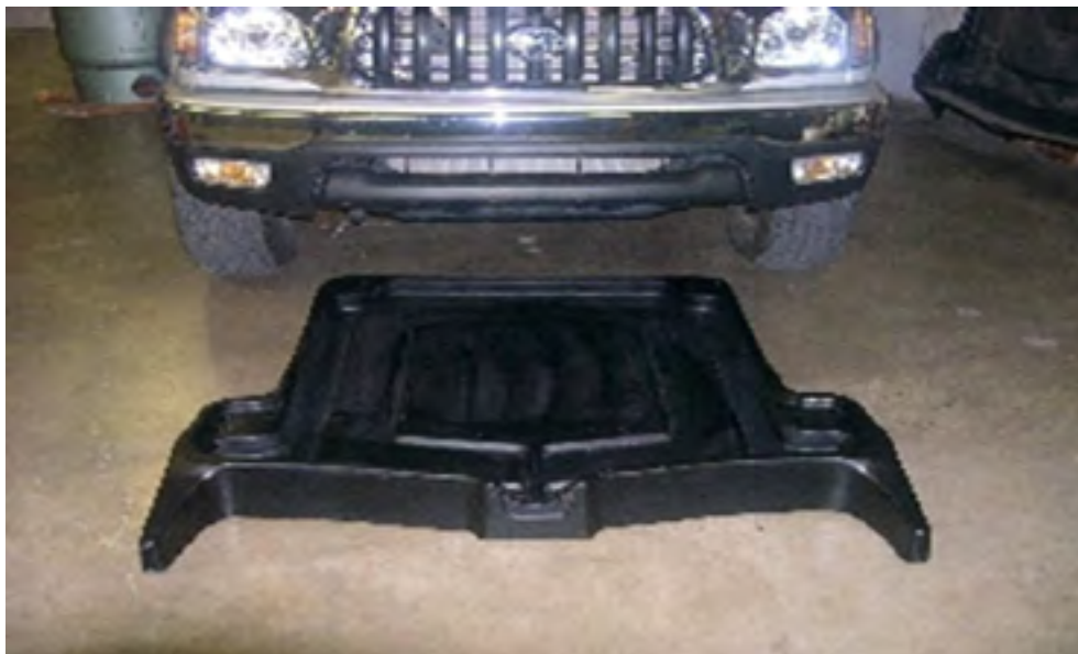
Figure 3.3. - Drip Pan for Capturing Spills and Drips During Engine Repair and Maintenance.
