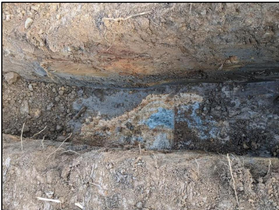
**Figure 33.** Photo of trench floor soil variations after dry terracotta pipe removal, plan view.
