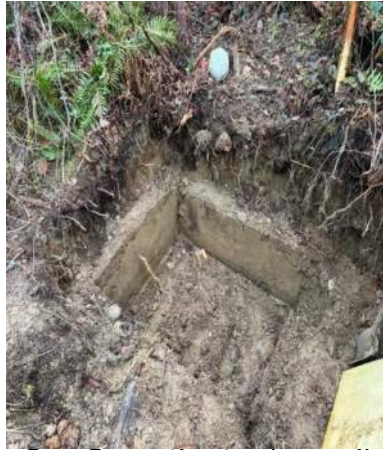
Over Excavation to observe if Groundwater is Mounding
