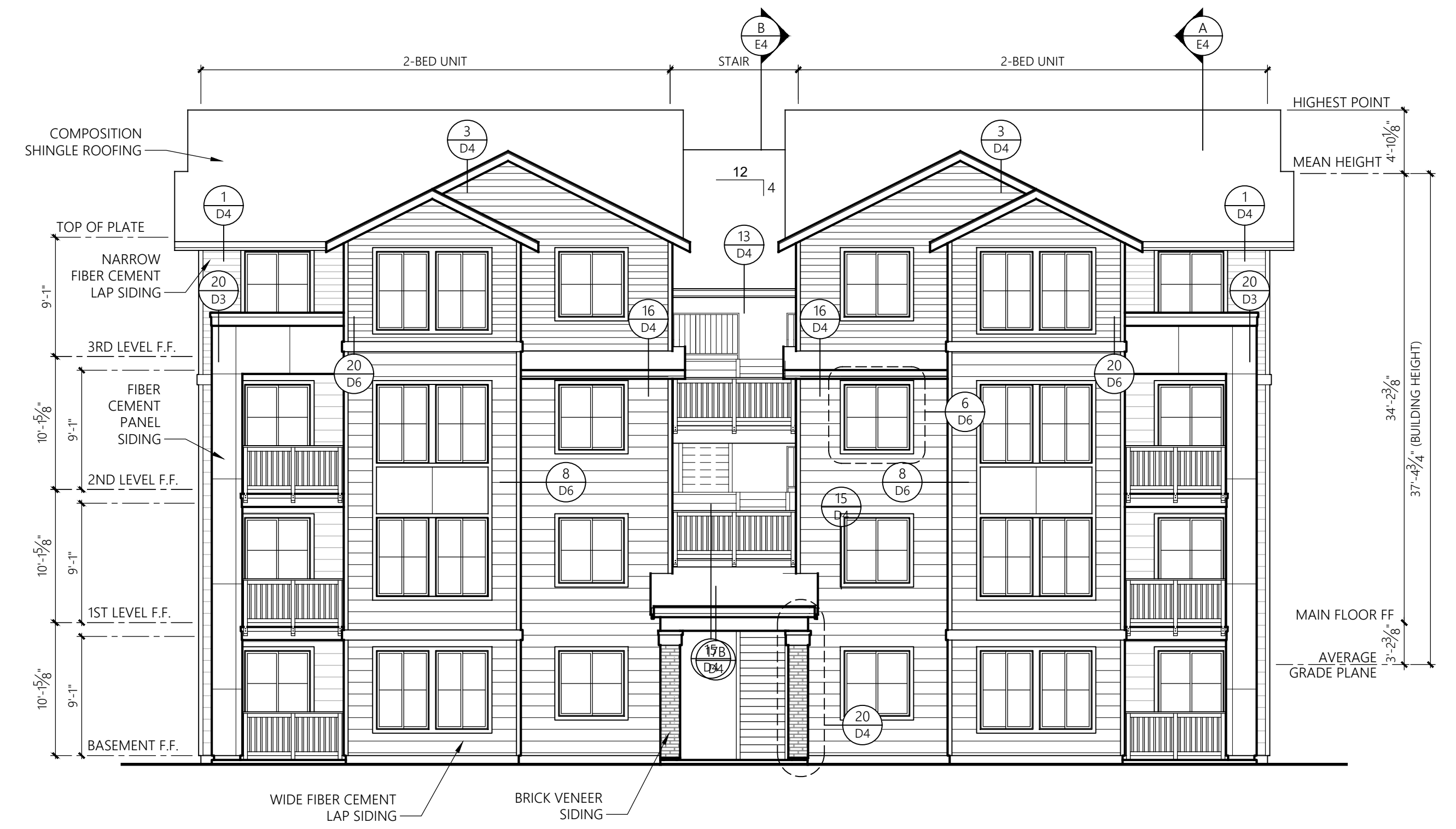
BUILDING B FRONT ELEVATION 1/8" = 1'-0"
