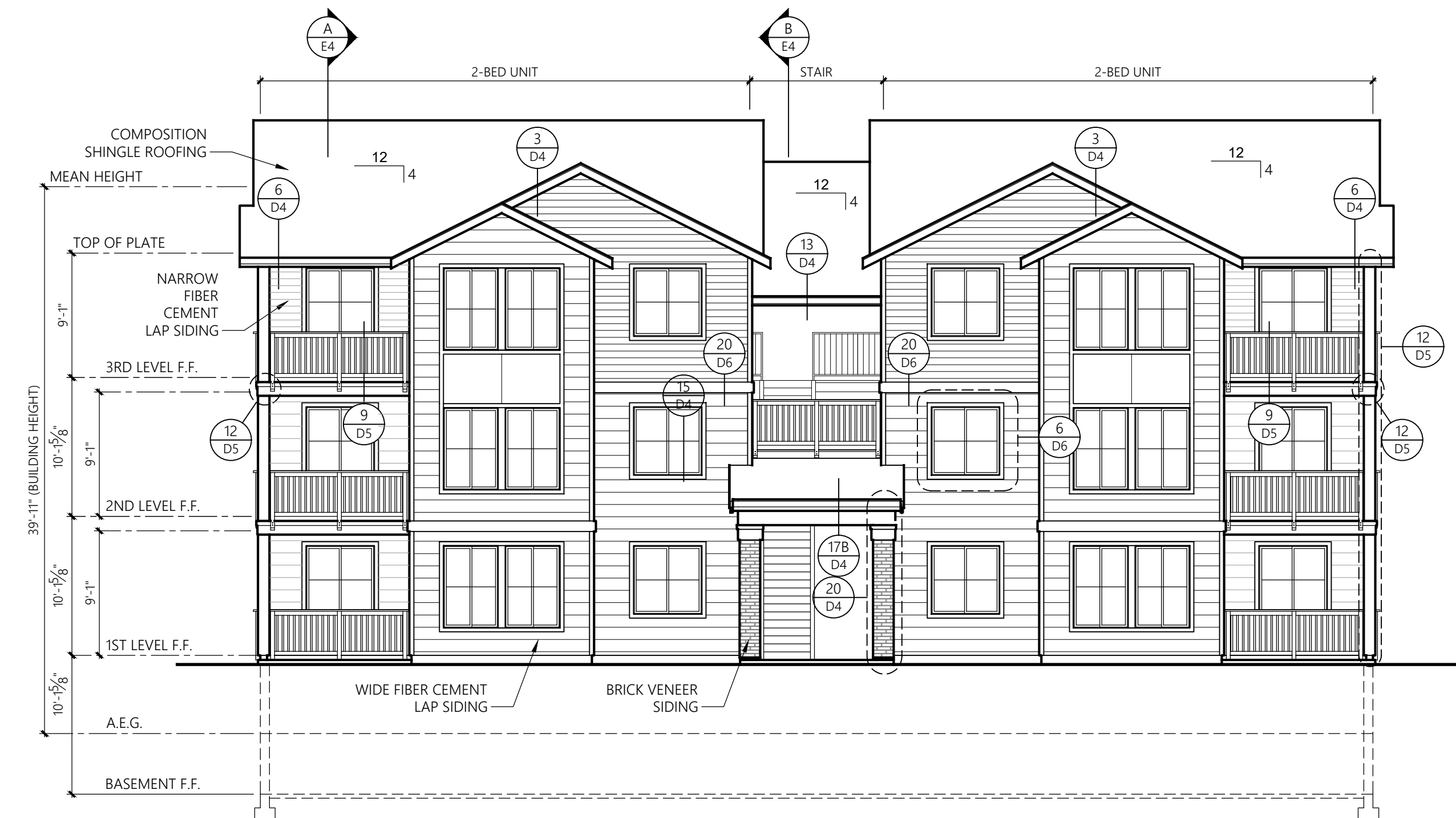
BUILDING B REAR ELEVATION 1/8" = 1'-0"
