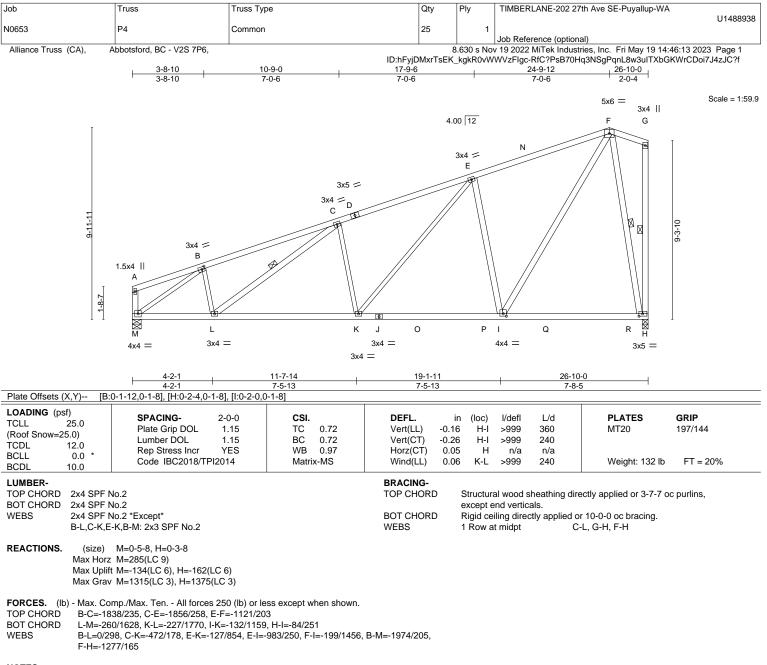
Wind: ASCE 7-16; Vult=115mph (3-second gust) Vasd=91mph; TCDL=4.2psf; BCDL=5.0psf; h=30ft; Ke=1.00; Cat. II; Exp B; Enclosed; MWFRS (envelope) gable end zone; cantilever left and right exposed ; end vertical left and right exposed; Lumber DOL=1.33 plate grip DOL=1.33
