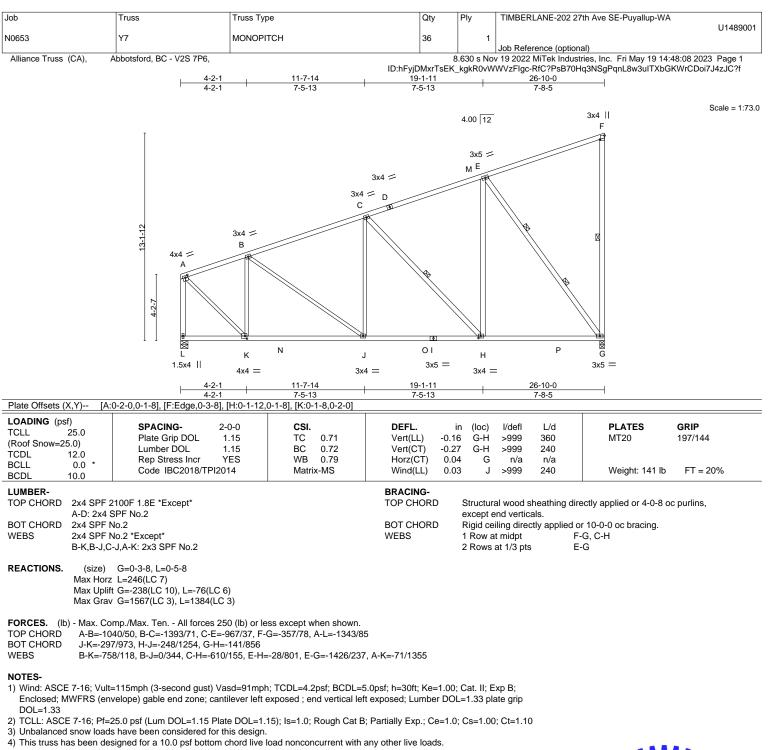
5) \* This truss has been designed for a live load of 20.0psf on the bottom chord in all areas where a rectangle 3-6-0 tall by 2-0-0 wide will fit between the bottom chord and any other members, with BCDL = 10.0psf.
