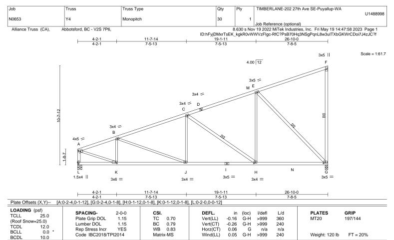
LUMBER-BRACING-2x4 SPF 2100F 1.8E \*Except\* TOP CHORD TOP CHORD Structural wood sheathing directly applied or 3-0-7 oc purlins, A-D: 2x4 SPF No.2 except end verticals. BOT CHORD 2x4 SPF No.2 BOT CHORD Rigid ceiling directly applied or 10-0-0 oc bracing. WEBS 2x3 SPF No.2 \*Except\* WEBS 1 Row at midpt F-G, C-H, E-G F-G,C-H,E-G,A-L: 2x4 SPF No.2
