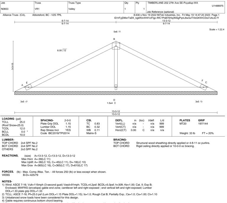
5) This truss has been designed for a 10.0 psf bottom chord live load nonconcurrent with any other live loads.
