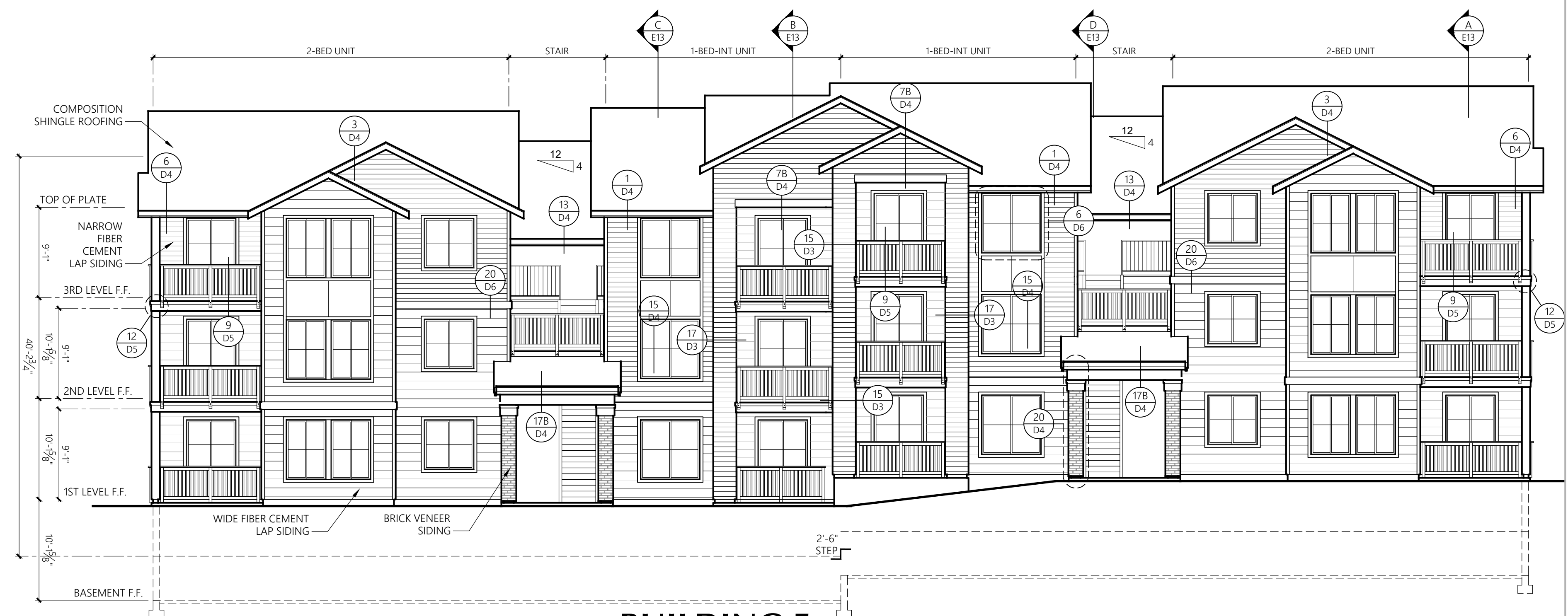
BUILDING F REAR ELEVATION 1/8" = 1'-0" ELEVATION SCHEME 1
