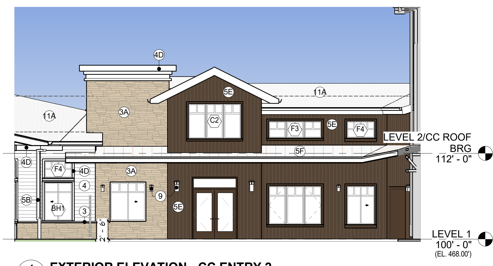
4 EXTERIOR ELEVATION - CC ENTRY 2 A3.2 1/8" = 1'-0"
