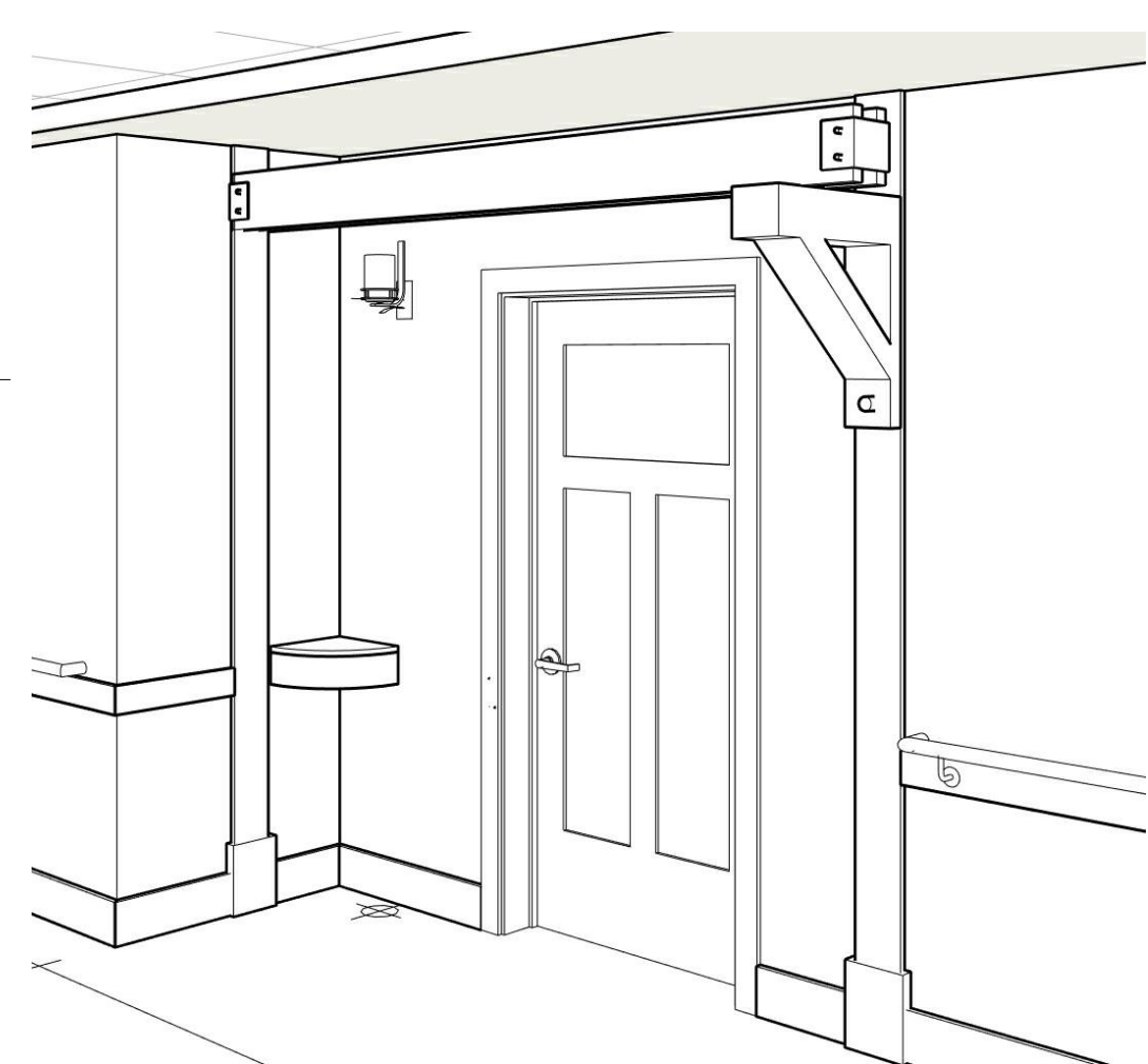
6 PILASTER DETAIL @ UNIT ENTRY A10.4 3" = 1'-0"
