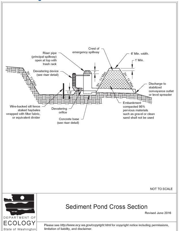
Figure II-3.30: Sediment Pond Riser Detail
