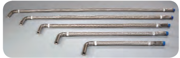
24", 36", 48", 60", 72" hose lengths. Rated working pressure 175psi, optional 300psi. Elbow model.
