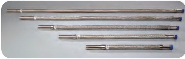
24", 36", 48", 60", 72" hose lengths, Rated working pressure 175psi, optional 300psi. Straight model, Standard 1" I.D., optional 1 1/4" I.D.
