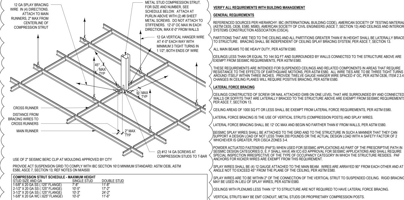
NOTE: FOR DOUBLE STUD, ATTACH WEB TO FLANGE WITH #6 SCREW @ 18"OC
