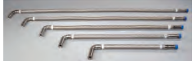
24", 36", 48", 60", 72" hose lengths. Rated working pressure 175psi, optional 300psi. Elbow model. Standard 1" I.D., optional 1¼" I.D. Model #: see page 5.
