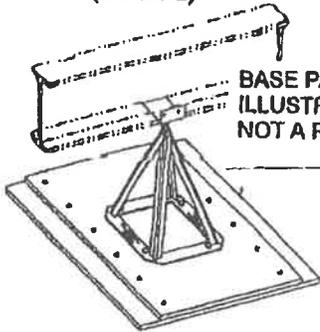
BASE PADS ARE SHOWN FOR ILLUSTRATION ONLY AND ARE NOT A PART OF THE PIER APPROVAL
