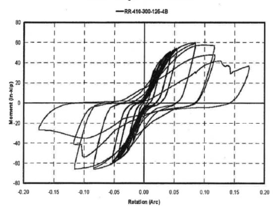
Secant stiffness at 0.095 rad > 500 in-kips per radian Maximum rotational capacity > 0.12 radians
