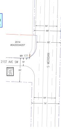
SPLICE SPARE FIBER TO THE SITE AT MH 177 FROM THE 144CT[A25NW] CABLE IN THE RANGE OF LPU10, 819-822. THE ENGINEER WILL PICK FIBERS AND SPLICE THEM TO 144CT [HR22] CABLE AND COUNT WILL FALL THROUGH MH 178 TO MH 180.
