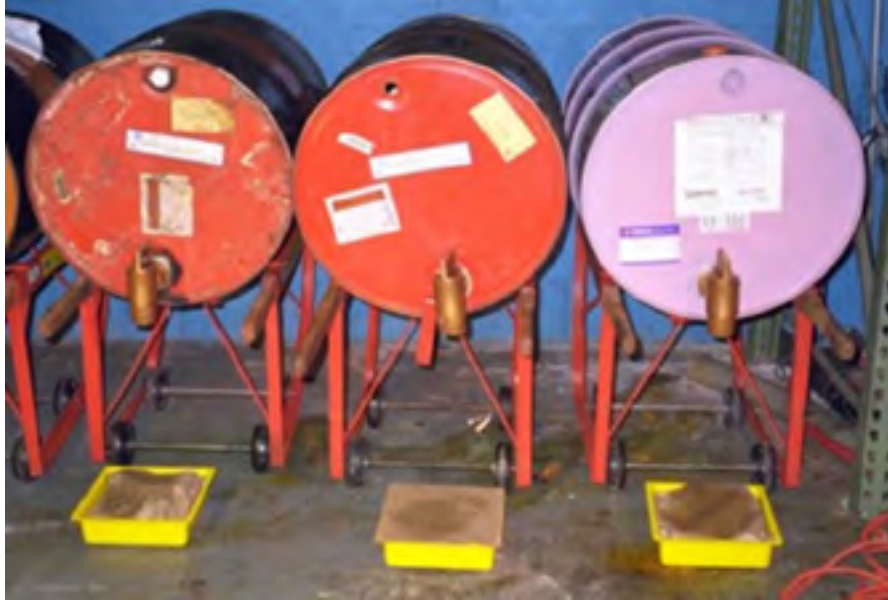
Figure 4.18. - Mounted Containers with Drip Pans.
