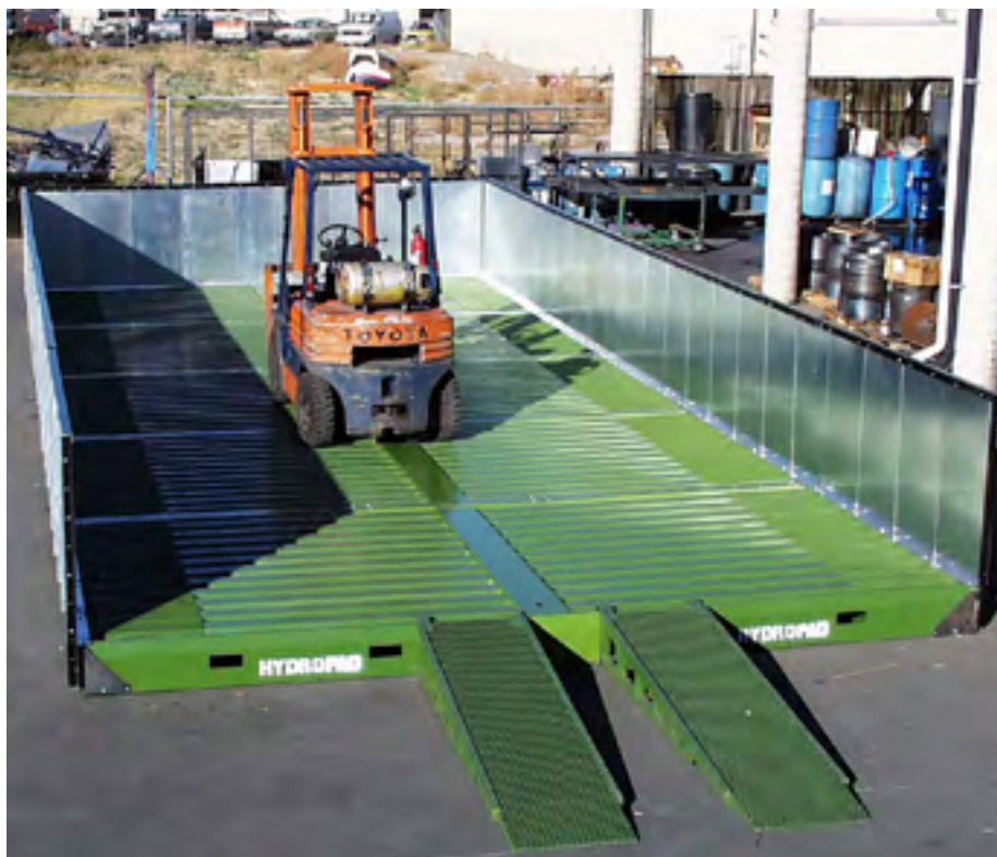
Figure 4.2. - Uncovered Washing Area for Tools, Engines, Equipment, and Portable Objects, with Drains to a Sanitary Sewer, Process Treatment, or a DeadEnd Sump.
