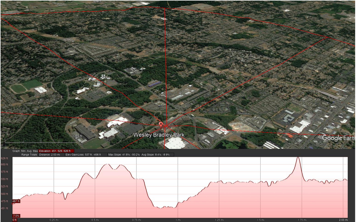
Figure 5: Southeasterly wind, escarpment is not an isolated feature therefore K_{zt} = 1.00
