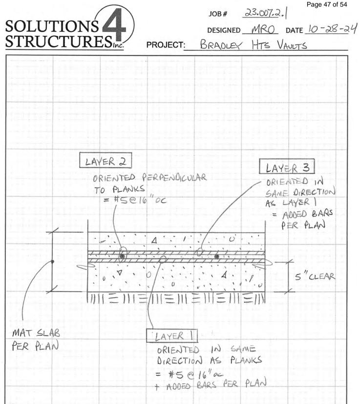
SLAB REINFORCEMENT PLACEMENT
