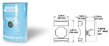
The service disconnect switch is used to temporarily disable the fire suppression system. One switch is installed on each of the two release circuits between the SIGA-REL and the RELA-EOL end-of-line relay. Opening the Service Disconnect Switch allows the fire alarm system to be tested without activating the fire suppression system. The operation of this switch causes a trouble signal at the control panel.
