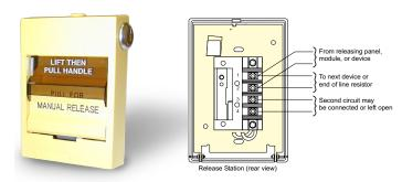
The manual release station is a normally-open, dry contact signal initiating device. The 276A-REL is a single-action station that requires the user to pull the release handle to initiate the release of a fire suppression agent. The 278A-REL (shown) is a double-action station that requires the user to raise the upper door, then pull the release handle to initiate the release.
