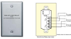
The End-of-Line Relay facilitates the connection of a non-polarized releasing solenoid to a supervised, polarized releasing circuit. One relay is required per release solenoid.
