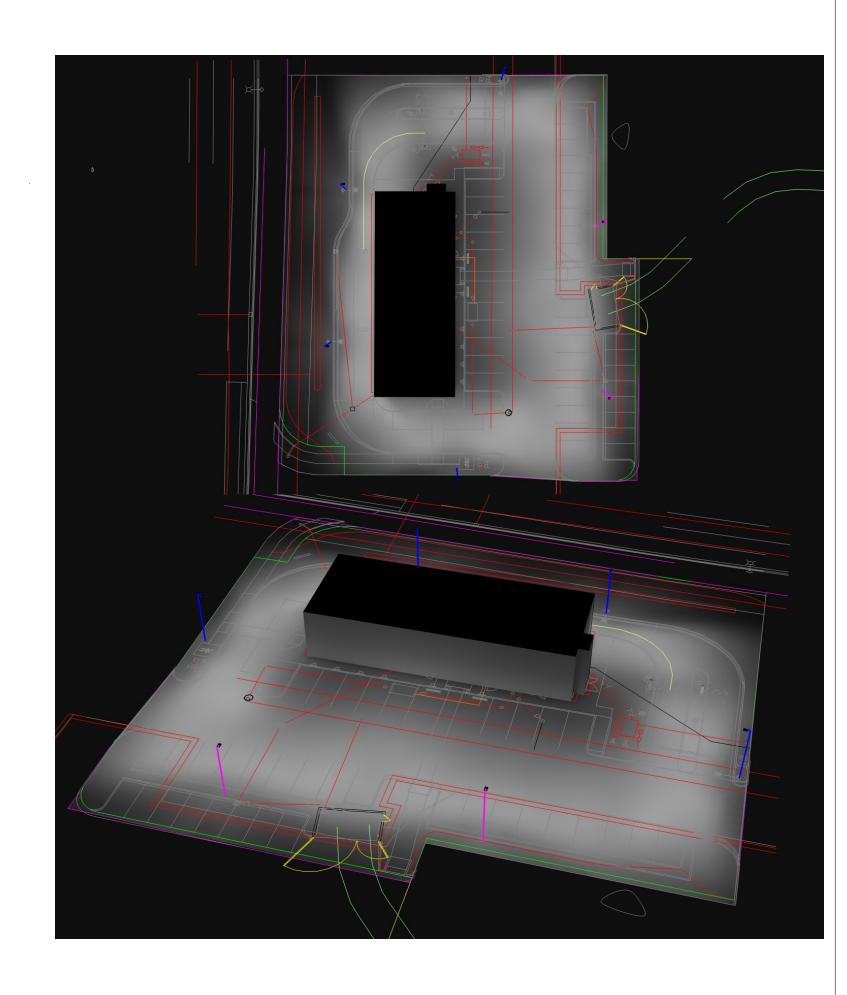
Pole Fixtures Are Full Cutoff Tilt=0 Calculation Grids Are At Grade Pole Light Mounting Height=21ft (18' Pole + 3' Base)
