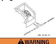
An uninsulated section of a single conductor should not be looped around the terminal and serve as two separate connections. The wire must be severed, thereby providing supervision of the connection in the event that the wire become dislodged from under the terminal. Failure to sever the wire may render the device inoperable risking severe property damage and loss of life.
