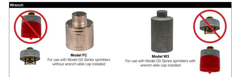
Fully insert the Model W3 wrench over the cap until it reaches the bottom of the cup, or the Model FC wrench over the sprinkler until the wrench engages the body. Do not wrench any other part of the sprinkler/cup assembly. The Model W3 and FC wrenches are designed to be turned with a standard 1/2" square drive. Tighten the sprinkler into the fitting after applying a PTFE based thread sealant to the sprinkler's threads. Recommended installation torque is specified in Table J.
