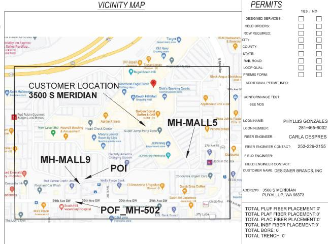
NARRATIVE:THIS PROJECT WILL PROVIDE CMS SERVICE TO 3500 S MERIDIAN. EXISTING 24 FIBER CABLE FROM POF\_MH-502TO MH-MALL9 IN EXISTING CONDUIT. EXISTING 24 FIBER CABLE FROM MH-MALL9 TO POI IN EXISTING CONDUIT. EXISTING 24 FIBER CABLE FROM POI TO MH-MALL5 IN EXISTING CONDUIT. EXISTING 24 FIBER CABLE FROM MH-MALL5 TO CUSTOMER MPOP IN EXISTING CONDUIT.
