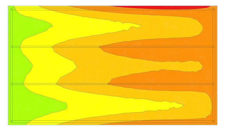
D + L + Storage: Max Soil Bearing Pressure Plan - 1
