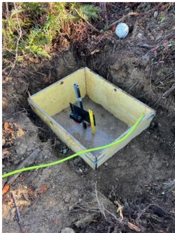
Pressure Transducer Drawdown Test
