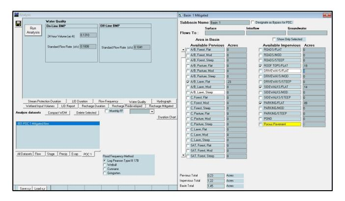
The original stormwater report has an offline flow rate of 0.1050 CFS. The new design has a resulting offline flow rate of 0.1041. The existing Biopod is sized for a flow rate of 0.128 CFS. Therefore, the water quality system is still adequately designed.
