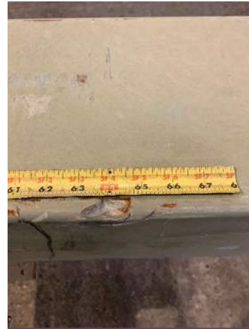
(b) Casing Gouge (Approx. 1/8" Deep)
