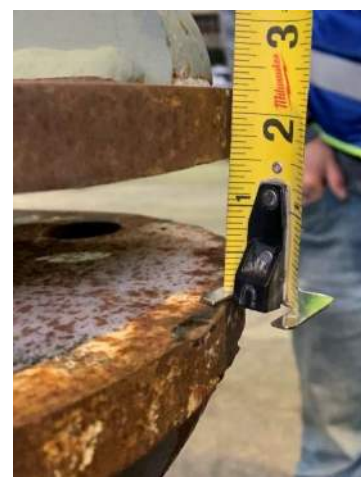
(f) Lug Measurement after Repair
