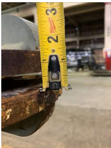
(e) Lug Measurement before Repair
