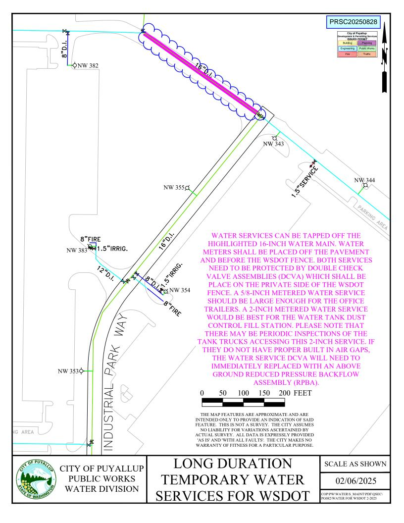
Prior to tapping the new water services, the contractor, in the presence of the City Inspector or City Water Department, shall determine the location of the proposed tap and the tap location of the future 8" water service to serve the future WSDOT weigh station. Moreover, the proposed 2" service shall be tapped at least 2 feet from the existing, adjacent 2" tap installed under permit PRSC20250218.
