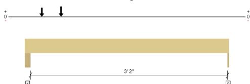
Drawing is Conceptual. All locations are measured from the outside face of left support (or left cantilever end). All dimensions are horizontal (typ.).
