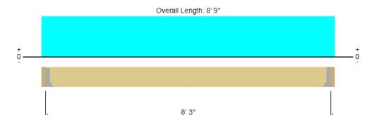
Drawing is Conceptual. All locations are measured from the outside face of left support (or left cantilever end). All dimensions are horizontal (typ.).
