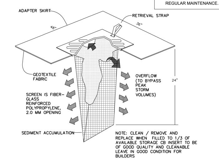
**DETAIL CBI-1 CATCH BASIN INSERT FOR TRASH & DEBRIS**
