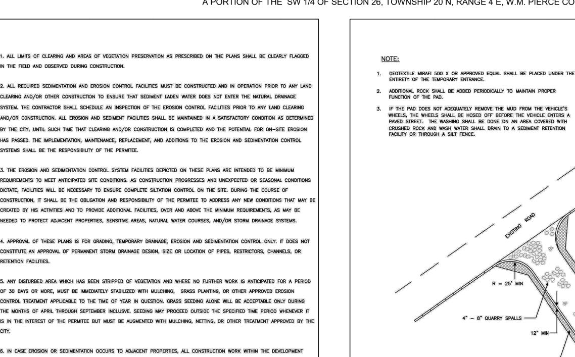
GRADING, EROSION, AND SEDIMENTATION CONTROL NOTES
